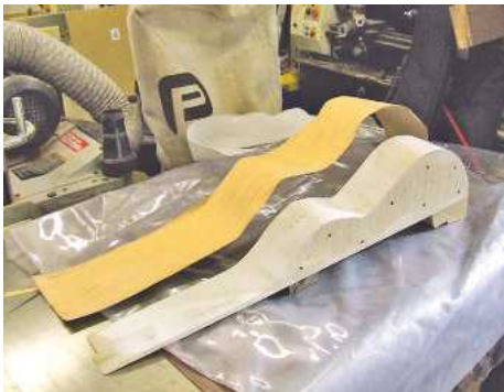
▲ Pic.13 Once dry, remove the piece from the bag and slip off the former – wax the former to ensure glue won't stick to it
